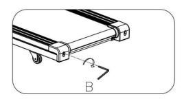
3. Over time the **Running Belt** will **loosen**. To tighten the belt turn the Left & Right side adjustment bolts one full turn clockwise, check the tension of the belt. Continue this process until belt is at the correct tension. Make sure to adjust both sides equally to ensure correct belt alignment. Refer to figure C.
